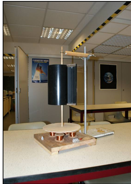
The completed Savonius generator (©ESEU)
