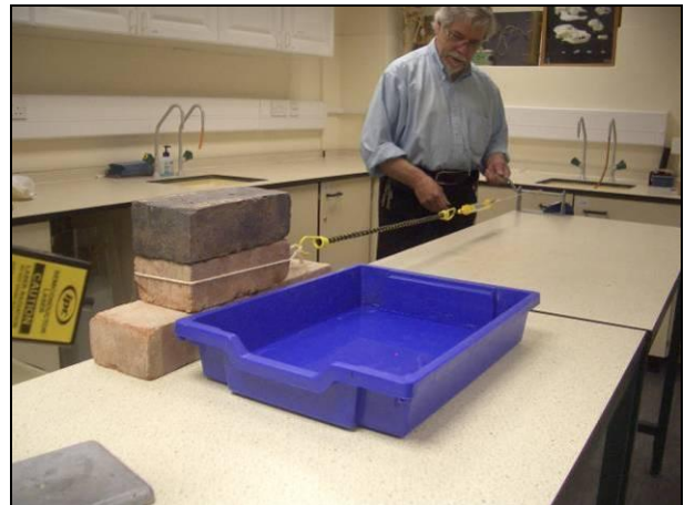
Brickquake pulled by a winding mechanism (©ESEU)
