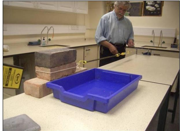
Brickquake pulled by a winding mechanism
