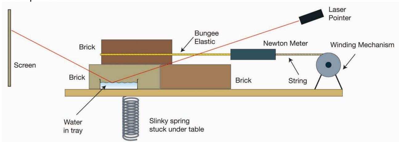
Diagram of brickquake apparatus (©ESEU)
