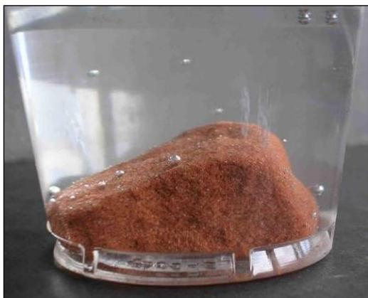
Figure 3: Sandstone 'bubbling' in a plastic beaker
